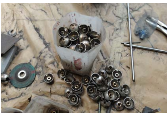
Fig.28. The manufacturing of specially designed clamps and problem solving fixing to hold small glass spheres © Tomasz Urbanowicz
